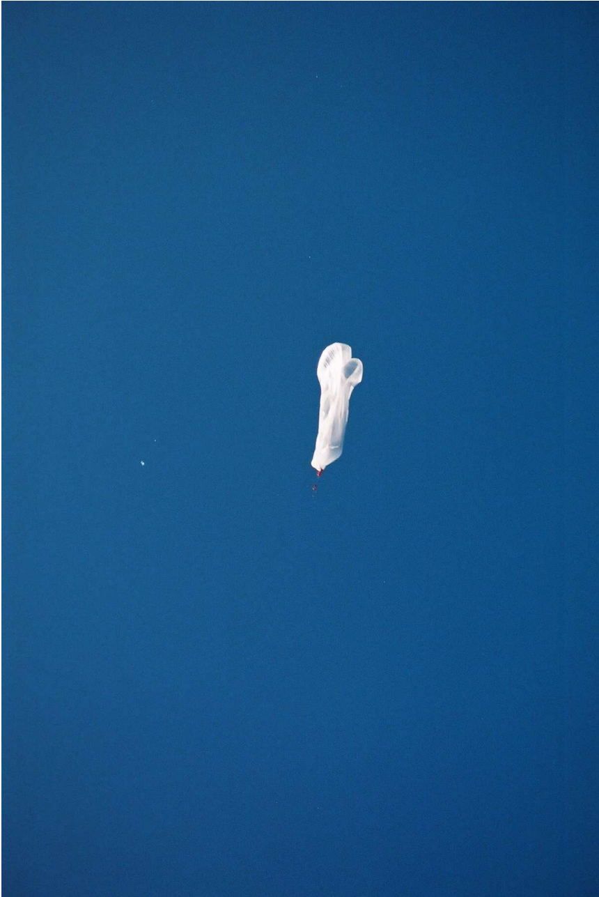
Fig. 4. 28000 cubic foot balloon which was fabricated in GS workshop. Note, the balloon is 100' tall.
