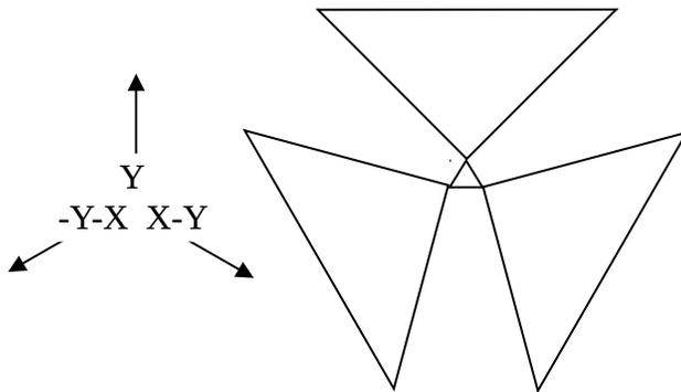
Figure 2. Solar Sail Spacecraft Vehicle Axis Definition.
