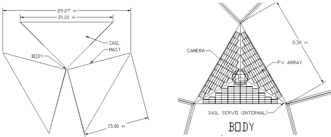
Figure 5 Solar Sail Vehicle dimensions
